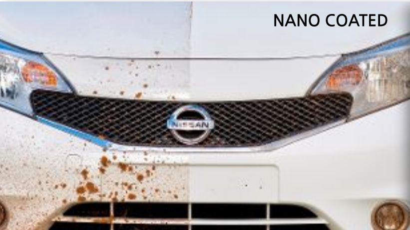
DIRT BOUNCING OFF HYDROPHOBIC NANO COATED MATERIAL
